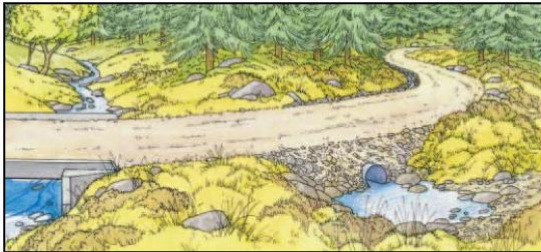
Above – Example culvert and filter zone.
