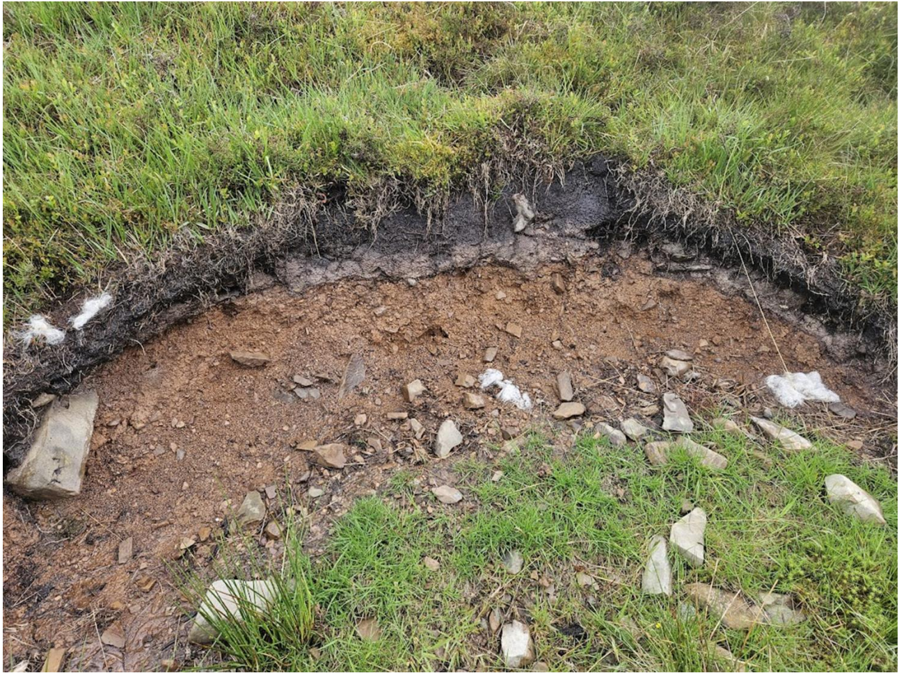
Ironpan soil (4) exhibiting Eg horizon underlain with thin Bf ironpan above ocherous Bs horizon
