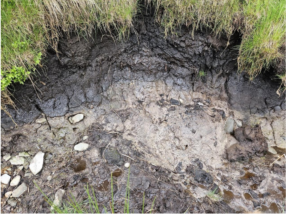
Peaty Gley with peat phase (6p) mineral horizon displaying complete reduction of iron due to long term waterlogging
