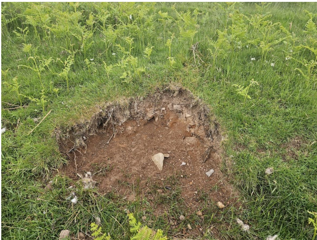
upland type (1u) exhibiting uniform brown colours but superficial gleying in the A horizon. Typical vegetation of bracken stands / acid grassland
