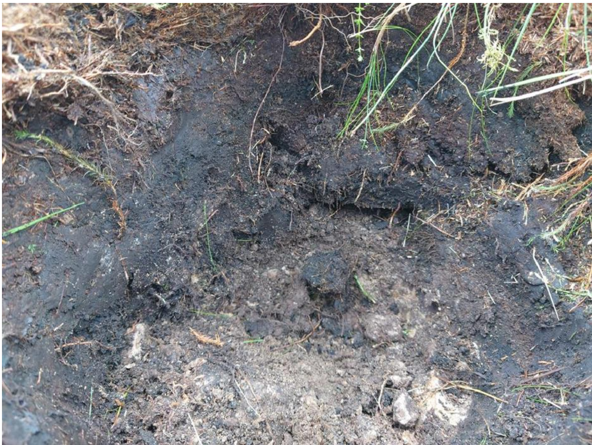
Peaty ranker – organic surface horizon underlain by very thin gleyed mineral horizon then solid parent material.
